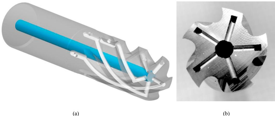
Figure 2: Internal structure of a 5ME BlueZone™ milling cutter: (a) internal structure schematic; (b) a cross section cut-off in the front [5]
