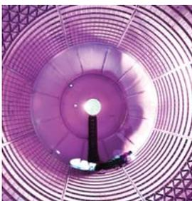
A technician inside the SLS liquid oxygen tank completes welds to plug holes left by a robotic welder. NASA engineers are now conducting hydrostatic testing on the tank. Read more about this and other core stage hardware on page 30. ■
