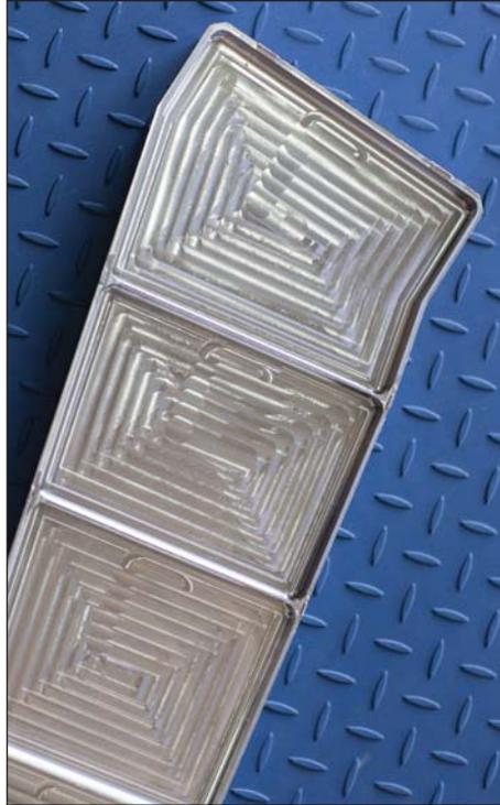
**Lockheed Martin Ti6Al4V structure component. Utilizing 5ME cryogenics, cycle time was reduced by 52 percent and piece cost reduced by 30 percent.**
